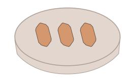
Polished, epoxy grain mounts of separate crystal alliquots prepared for Raman analyses
