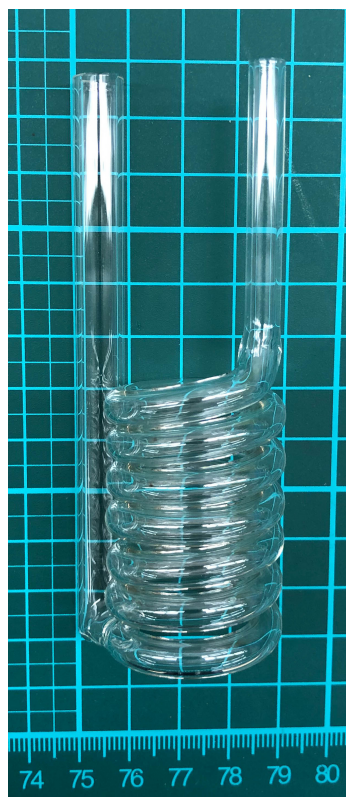
Figure 2. Compact borosilicate glass coil trap, consisting of a 9 mm o.d. \times 7 mm i.d. inlet downtube (on the left), connected to a tightly coiled 6 mm o.d. \times 4 mm i.d. section with subsequent outlet tube. The scale on bottom is in centimeters.
