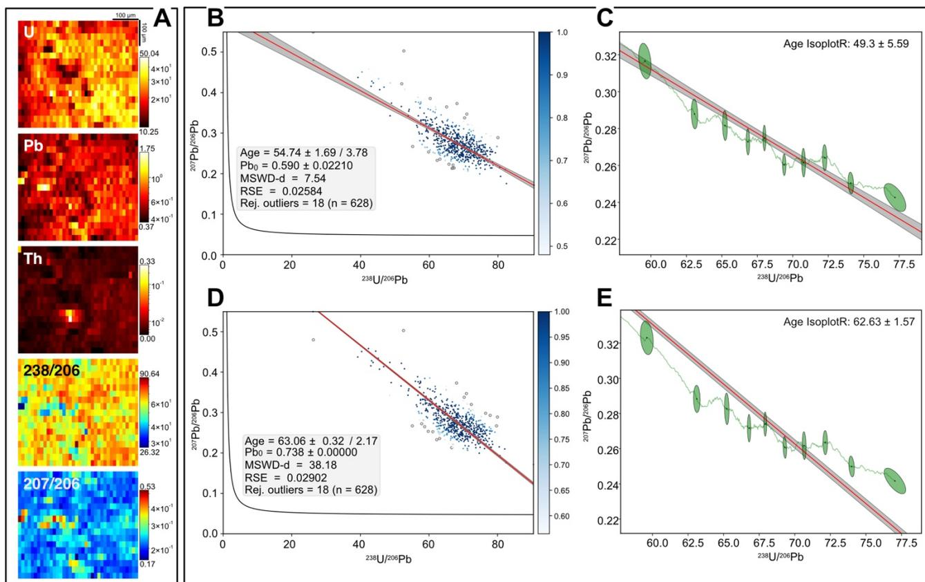
455 **Figure 2: A: Element concentrations in ppm (U, Pb, Th) and  $^{238}\text{U}/^{206}\text{Pb}$ ,  $^{207}\text{Pb}/^{206}\text{Pb}$  isotopic maps obtained for one analysis of Duff**
