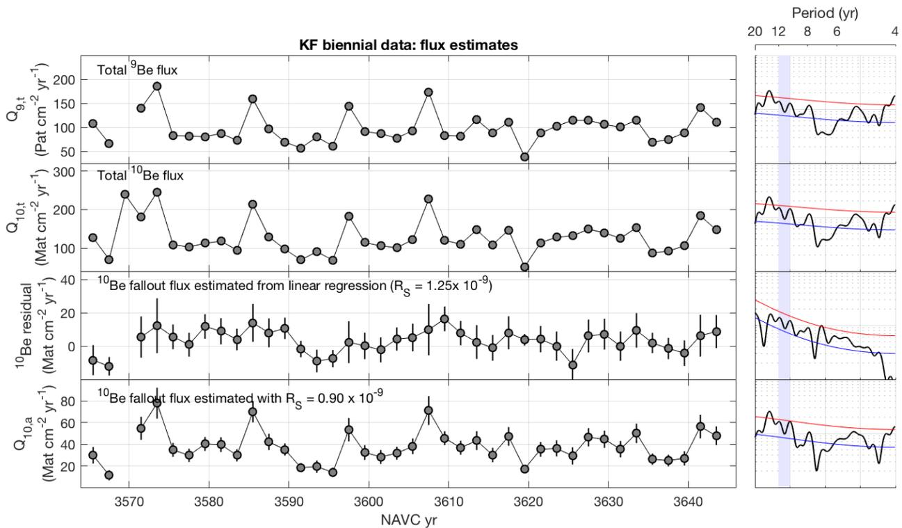
**Figure 15.** Be flux estimates for 80-year biennial record at KF. Total fluxes are calculated using the grain size - sediment density relationship shown in Figure 3. Fallout fluxes are estimated from two different assumed values of  $R_S$ ; see text for details. Error bars reflect propagation of uncertainty on Be isotope concentrations, but not on mass accumulation rates. Plot elements for MTM spectra are the same as in Figure 11.
