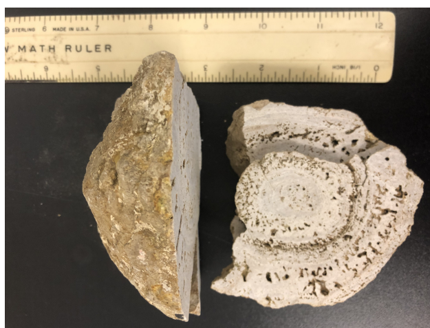
Figure 10. Hand specimen of a Barstow Formation tufa sample that is large enough to slab and share as a secondary LAcarb standard.
