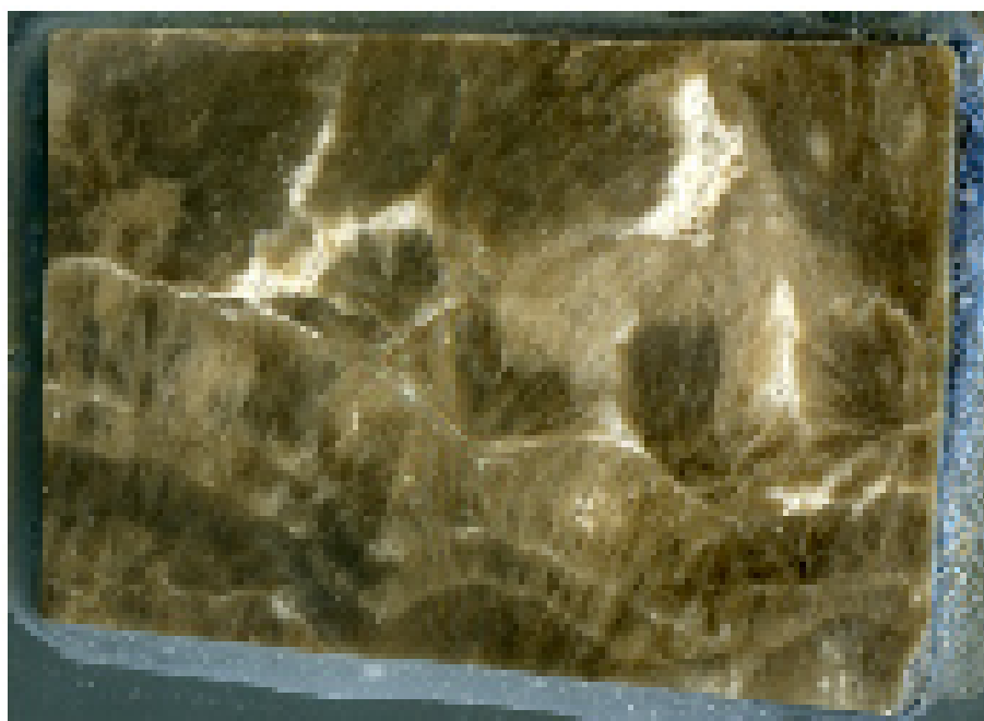
Figure 3. Polished slab from the Walnut Canyon Neptunian Dike sample used in this study to illustrate various tools for characterization. This is approximately 3 cm across. This is a similar size to that being distributed as a primary standard (Roberts et al., 2017). Note the variability of color from very dark to light brown, and white veins. The fibrous botryoidal texture is visible even at this scale, and complexities due to veins should be easily avoided when using this as a LAcarb standard.
