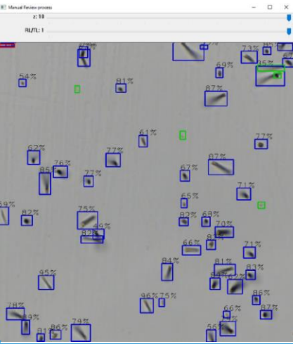
Figure 3: fission track recognition in muscovite (external detector). Blue squares indicate automatically recognized semi-tracks. The percentage displayed above every blue box indicates the confidence score for that particular group of pixels to be recognized as semi-track. The small fraction of unrecognized tracks ("false negatives") is manually indicated with green squares. Red squares indicate erroneously indicated tracks ("false positives"). The two track bars above the image indicate the possibility to compare different focal levels or change between reflected and transmitted light.
