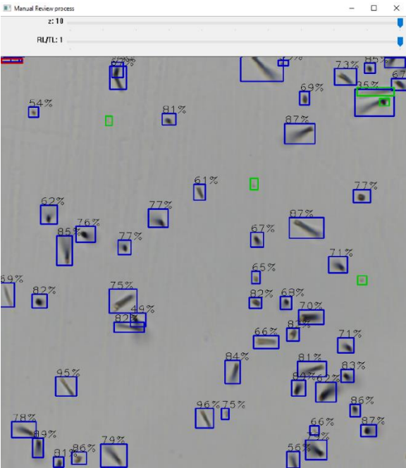
Figure 2: fission track recognition in muscovite (external detector). Blue squares indicate automatically recognized semi-tracks. The percentage displayed above every blue box indicates the confidence score for that particular group of pixels to be recognized as semi-track. The small fraction of unrecognized tracks (“false negatives”) is manually indicated with green squares. Red squares indicate erroneously indicated tracks (“false positives”). The two track bars above the image indicate the possibility to compare different focal levels or change between reflected and transmitted light.
