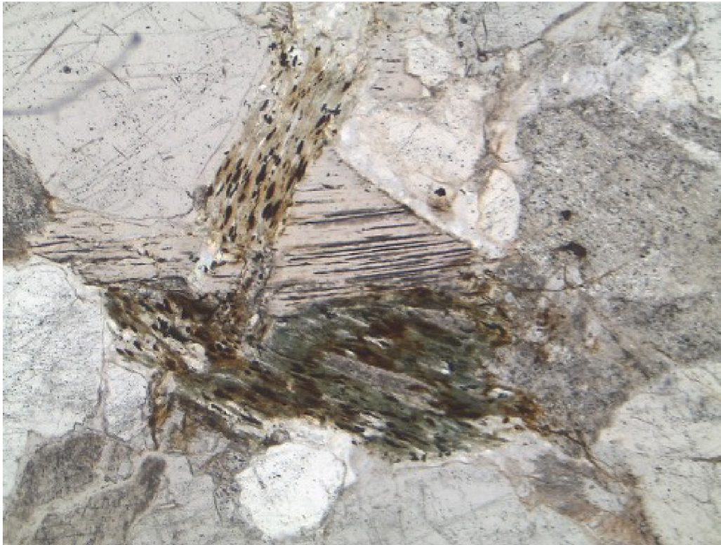
Fig.10: Microphotograph of a chloritized biotite in granite fragments closely associated to geodic fluorite (width ca. 1mm)
