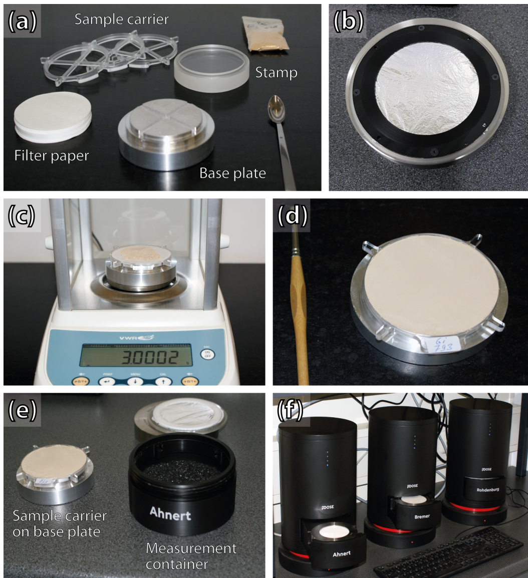
Figure 1. Photos showing the \mu Dose-devices and equipment: (a) Sample carrier and equipment for sample preparation. (b) Scintillator unit with silver foil. (c) High-precision balance used for weighing 3.00 g of sample material. (d) Prepared sample on a sample carrier with a diameter of 70 mm. (e) Prepared sample material and measurement container. (f) Three \mu Dose-devices installed in the Giessen Luminescence Laboratory.
