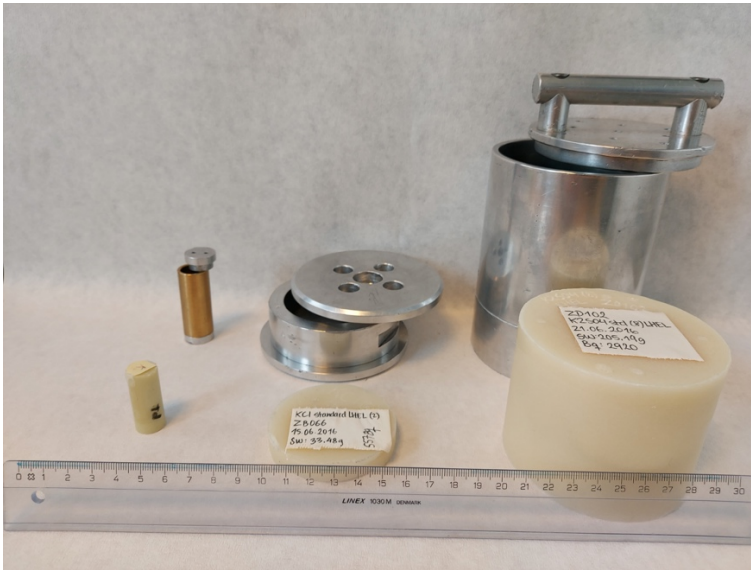
Fig. B2. Samples mixed with wax and casted in three different geometries (Photo kindly provided by Vicki Hansen, DTU).
