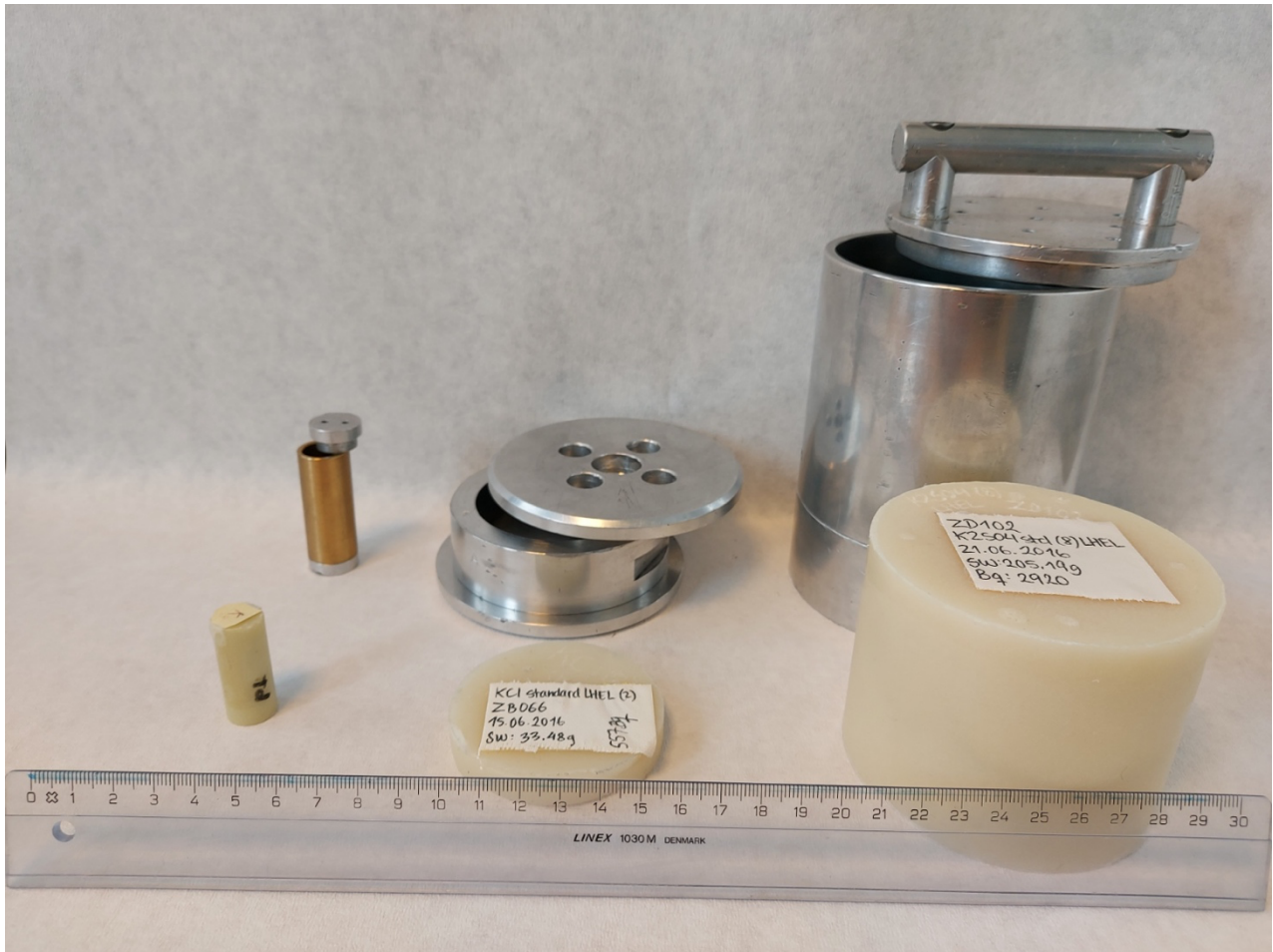
510 Fig. B2. Samples mixed with wax and casted in three different geometries (Photo kindly provided by Vicki Hansen, DTU).
