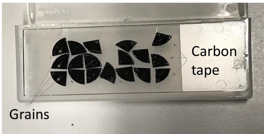
Figure S1: Grains mounted for \mu XRF/ \mu XANES measurements. Grains are attached with carbon tape to avoid movement.
