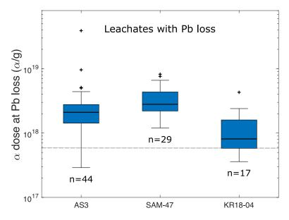
Figure 11. Box plot diagram showing alpha dose distribution for leachates (L1, L2, and L3) affected by Pb loss. Data include both the 180 °C and 210 °C experiments. The gray dashed line highlights our best estimate for the minimum alpha dose required for Pb loss to occur. Each box shows the median value (black bar), the upper and lower quartiles (box), the minimum and maximum values (whiskers), and statistical outliers (plus marks).
