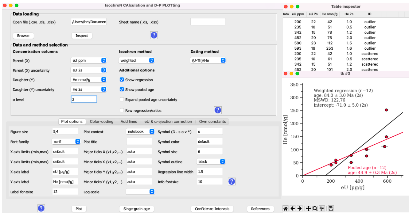
Figure 14. Main window of the Incaplot software (left), the table inspection tool (upper right) and an output D-P plot (lower right).
