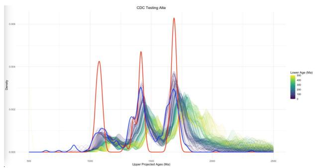
In this image, the red lines are the 7/6 ages of the concordant data population (all lines are a kernel density estimators using 15 Ma bandwidth). The other curves are CDC projections from various lower intercept points (the color reflects the lower intercept age) through the discordant data points and we show the distribution of those recalculated upper intercept ages. Importantly, the discordance dating age of 24 Ma is shown in the blue curve.
