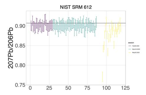
The beginning analyses of Run #3 do fall significantly outside of uncertainty of the accepted value. But these do not affect the samples or standards analyzed later during this session, and do not impact the trace-element data collected on the iCAP-RQ mass spectrometer. We have added text to the manuscript, and additional supplemental figures in the GitHub repo documenting this and further U-Pb data descriptions (reference in a revised version of the manuscript).
