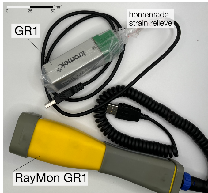
Figure 1. Kromek detectors used for our measurements (shown is the probe without the handheld tablet PC for the RayMon10 ® ). Both probes house a similar CZT detector. We wrapped the GR1 ® in a standard plastic bag and attached a home made strain relief to the GR1 ® to enable easier operation and retraction of the detector in the field.
