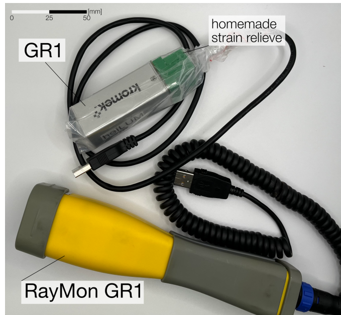
Figure 1. Kromek detectors used for our measurements (shown is the probe without the handheld tablet PC for the RayMon10 ® ). Both probes house a similar CZT detector. We wrapped the GR1 ® in a standard plastic bag and attached a home made strain relief to the GR1 ® to enable easier operation and retraction of the detector in the field.
