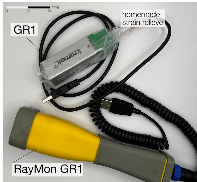
**Figure 1.** Kromek detectors used for our measurements (shown is the probe without the handheld tablet PC for the RayMon10<sup>®</sup>). Both probes house a similar CZT detector. We wrapped the GR1<sup>®</sup> in a standard plastic bag and attached a home made strain relief to the GR1<sup>®</sup> to enable easier operation and retraction of the detector in the field.
