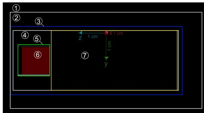
**Figure 2.** Geometry of the simulated CZT detector – image from *GEANT4* visualization. Legend: (1) Sediment matrix; (2) rubber coating; (3) aluminum shielding; (4) air; (5) plastic support; (6) CZT crystal; (7) electronic components. Information kindly provided by the Kromek Group plc.
