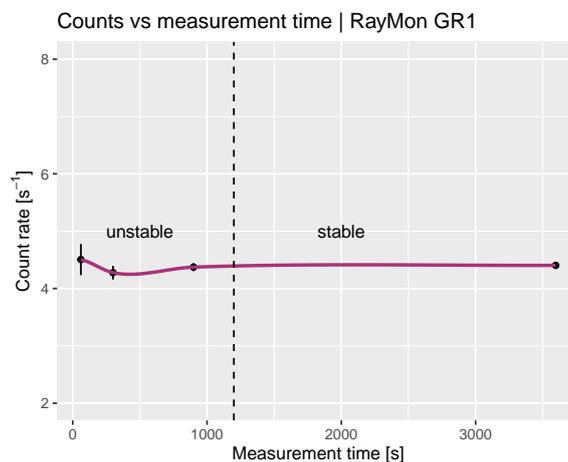
**Figure 7.** Sum of counts normalised to the measurement time recorded in the brick block at Archéosciences Bordeaux. After 20 min the average count rate does not change anymore within uncertainties. The plot scales depending on the settings of  $\eta$  (the energy threshold) and it was arbitrarily set to 200 keV for this graph.
