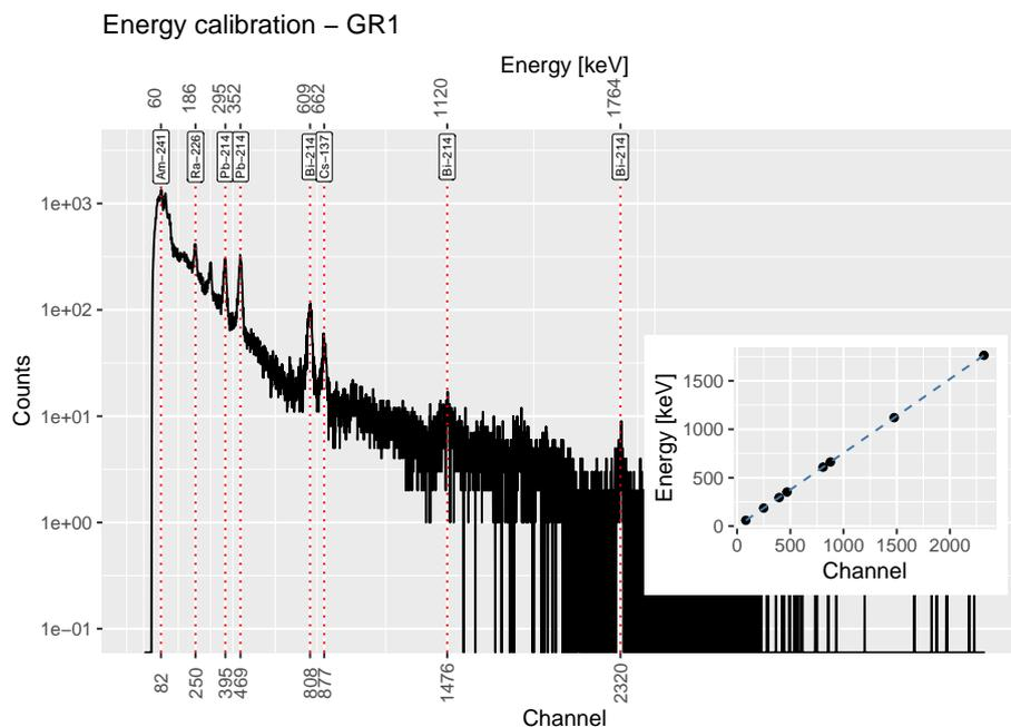
**Figure 4.** Energy calibration results for detector GR1. The main plot shows the raw spectrum with known  $\gamma$ -lines marked with dashed lines. The inset displays the calibration curve applied to all subsequently shown spectra. Peak positions were found to be similar for GR1 and RayMon GR1.
